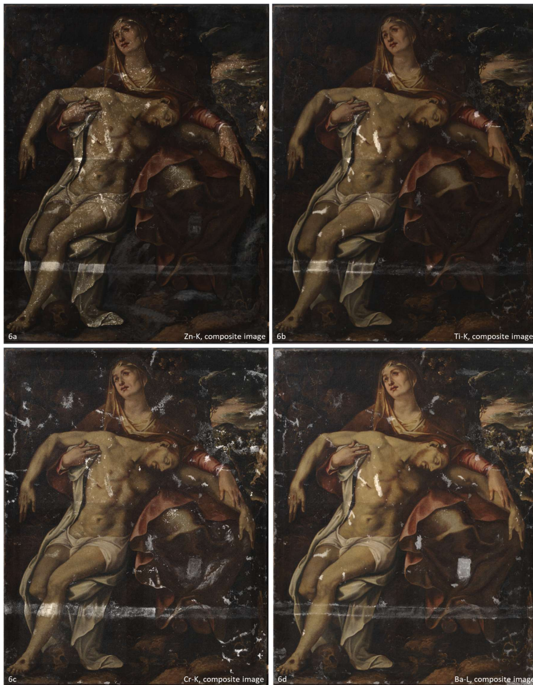
Figure 6. Areas with retouching with modern pigments: a) with zinc white, b) with titanium white, c) with chromium containing pigments, and d) with barium sulphate.
